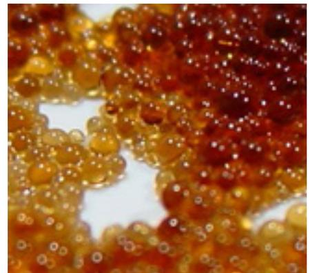
On contact with water, this sodium (which is non scale forming) exchanges with the calcium and magnesium in the water.
